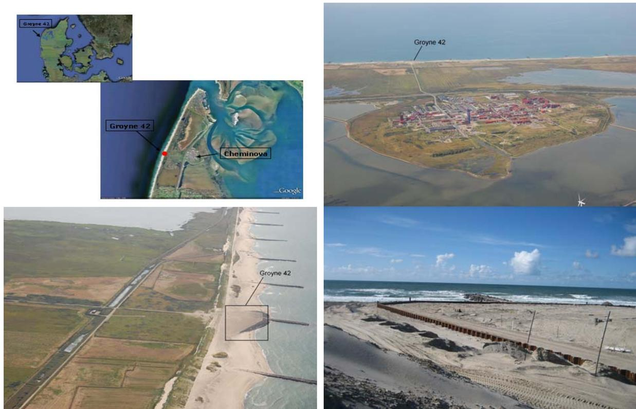
Figure 2. Photos of the location of the site in Denmark. The former chemical dumpsite is located right on the beach close to the North Sea. In the lower right photo is seen the iron sheet piling enclosing the contamination.
