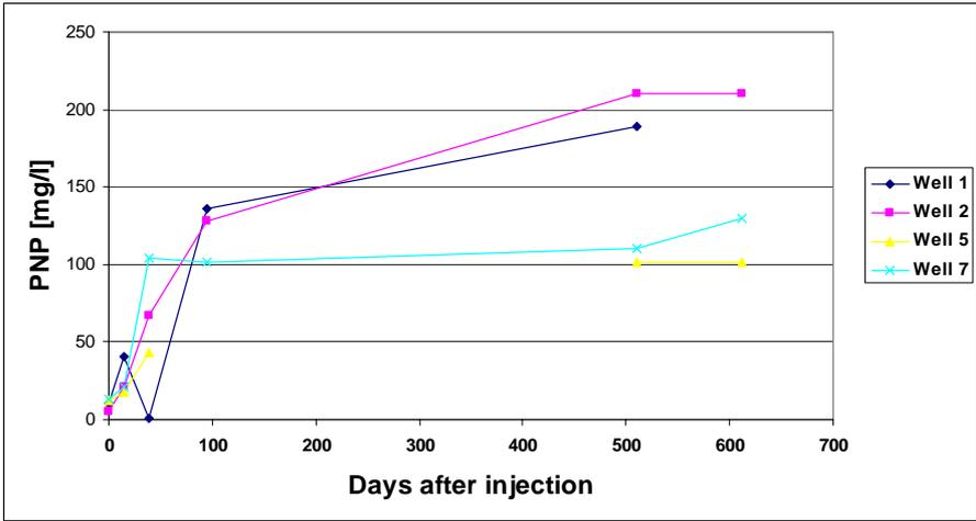
Figure 8. Concentration of the ethyl-parathion breakdown product “PNP” in the observation wells after injection with NaOH.
