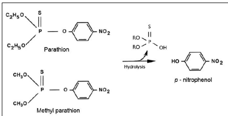
Figure 3. Chemical reaction showing the principle of the alkaline hydrolysis of organophosphorous pesticides.
