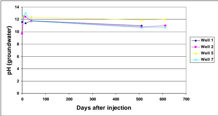
Figure 6. pH in the observation wells after NaOH injection
