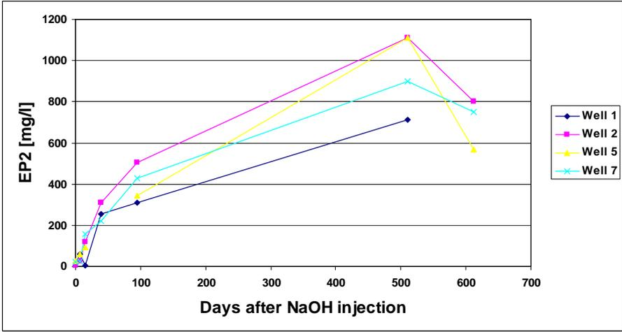
Figure 7. Concentration of the ethyl-parathion breakdown product “EP2” in the observation wells after injection with NaOH.
