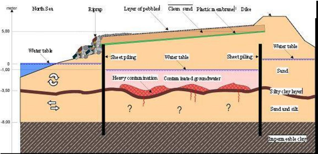
Figure 1: principle sketch of the enclosed site.
