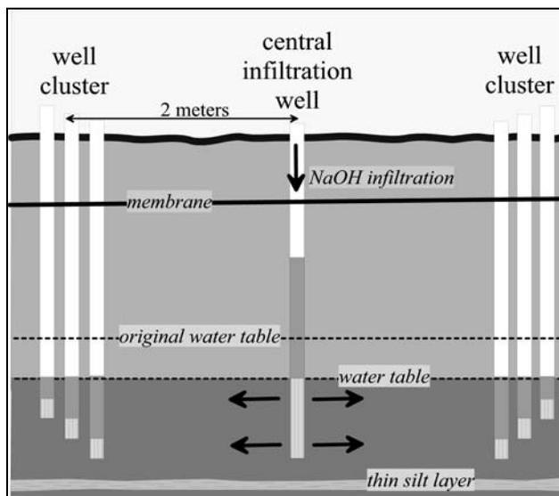
Figure 5: Design of field experiment with alkaline hydrolysis
